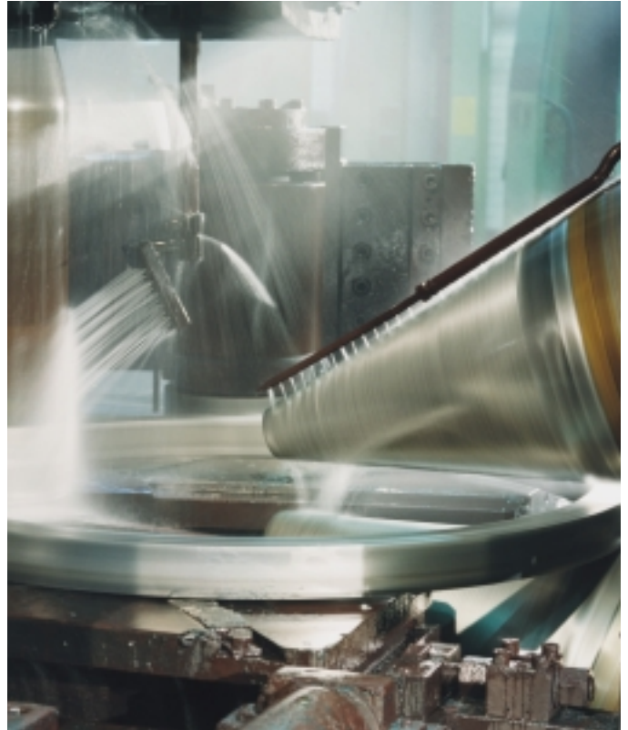
Ring Rolling Mill RAW 315.
