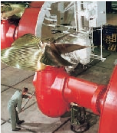
Rudder propeller, Lips Thrusters Drunen B.V., Drunen, The Netherlands
