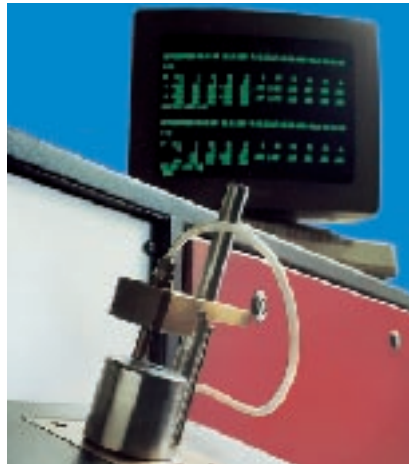
Spectral analysis of rolling elements
