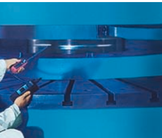
Fatigue test geared ring
