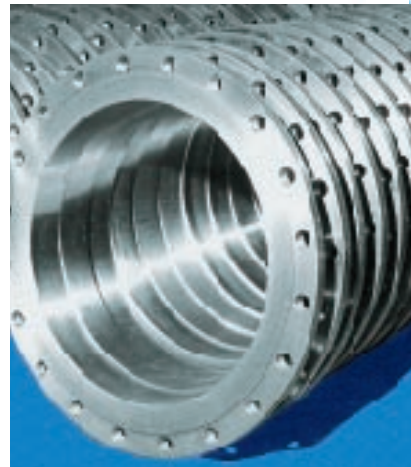
Finish-machined and drilled flange rings
