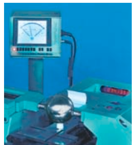
Routine test for rolling elements
