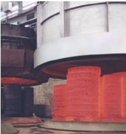
Bell-type annealing plant with 3 workstations
