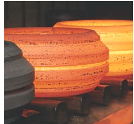
Profiled rings on the cooling bed
