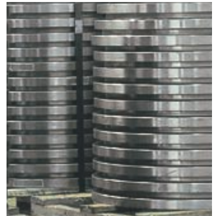
Profile rolled titan rings for aircraft jet engines
