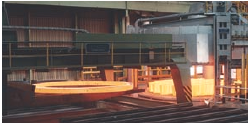
Bell-type annealing plant with manipulator for large ring diameters
