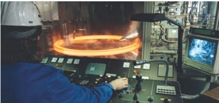
Control desk of the RAW 315 ring rolling mill
