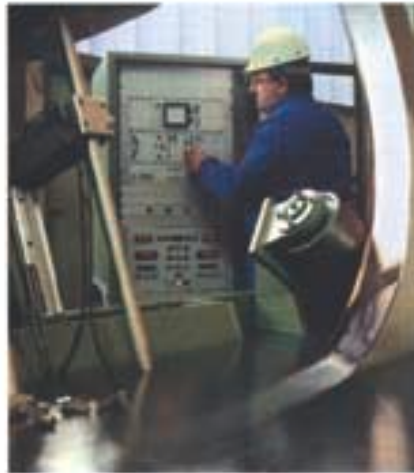
Ultrasonic testing of ring blanks.
