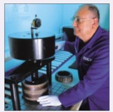
The Taper Bearing Units (TBUs), used on railway rolling stock are critical to the smooth running of any rail system. The refurbishment of railway bearings is a specialised task requiring expertise and specialised equipment. The quality of our workmanship is guaranteed and all refurbished TBU bearings leave the SKF Reliability Systems service centre fit for further service and carrying a full warranty.
