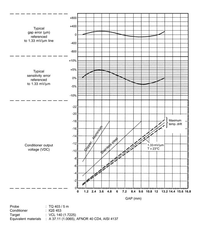
Note: In spite of its good dynamic response, the TQ 403 probe is essentially intended for displacement and not vibration measurement.
