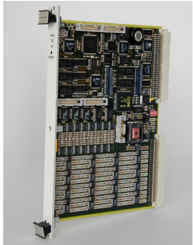
Figure 19. Parallel FFT Data Acquisition CMC-16.
