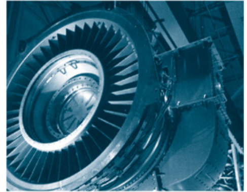
Figure 1. LM5000 derives from the CF-6 Aero Engine.
