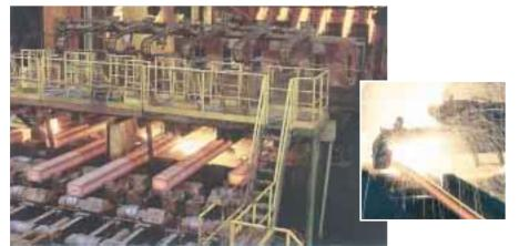
Continuous casting is an environment with high loads, high temperatures and low speed. The low speed makes bearing lubrication difficult since the lubricant can be pressed out instead of forming a film. The lubricant can also be washed out by the cooling system. Read about how we solved it.
