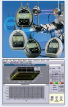
The readings from the Microlog are then processed within SKF PRISM<sup>4</sup> in the same way as those from PM5.
