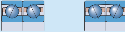
Static axial stiffness for two bearings arranged back-to-back or face-to-face – 719 .. D series
