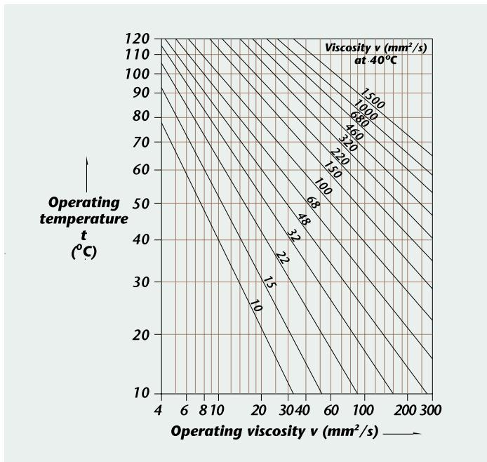
Using the operating temperature and nominal lubricant viscosity, the value for operating viscosity,  $V$ , is read off the horizontal axis.
