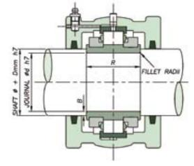
N.B. Width of recesses for standard bearings maybe different from that used for existing products. Please consult SRB Technical Services department for bearings suitable for other recess sizes.
