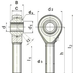
The international standard sets the dimensions of rods with spherical bearing assembled. It also specifies tolerances relative to the dimensions.
