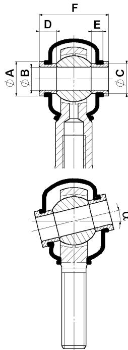
This protection completely conserves the rod-end bearing from any external attack:
