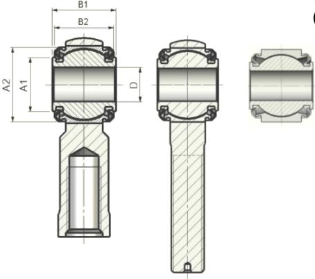
On request, we make sealed rod-end bearings, fitted with bellows.
