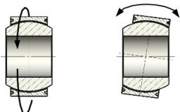
The spherical bearing's torque can be measured in relation to two perpendicular axes.
