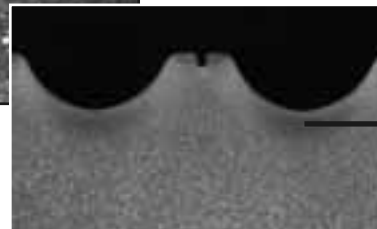
Profile of a rolled PSF Technology screw
