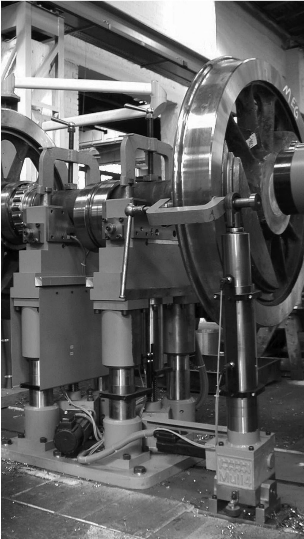
Surveying axles for rod locomotives, Hörmann Railway Technology, Germany
