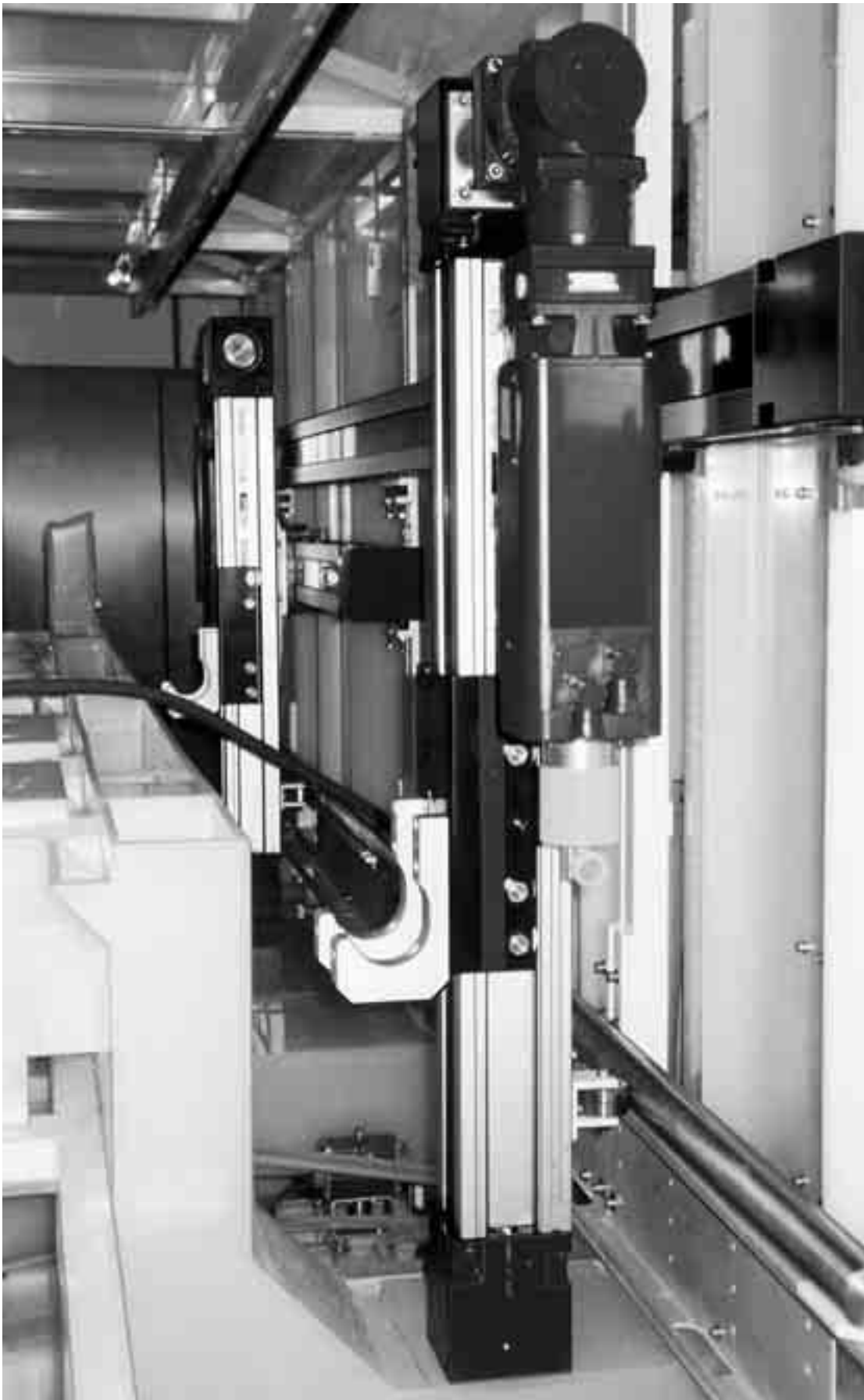
Automated 2-axis-handling of a cleaning system for semiconductor production in clean room. Astec GmbH in Berg, Germany.
