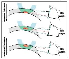
performance code 629 calls for a tighter rib/angle tolerance range, providing improved control of the rib/roller endcontact location.
