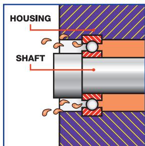
**A seal keeps contaminants out and lubricants in to protect and extend bearing life.**
