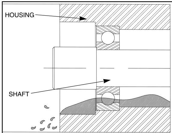
Without an oil seal . . . essential lubricant can escape through the bearing and . . . harmful dirt and foreign matter can enter.
