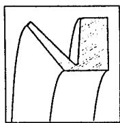
**VRS1** The standard design of the industry covers a shaft range of 0.11" to 79.53" (3 mm to 2000 mm).
