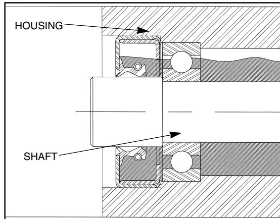
With a properly designed and fitted oil seal . . . the space between the housing and shaft is securely closed or sealed. Lubricant cannot escape . . . harmful dirt and foreign matter cannot enter.
