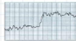
Poor race-to-face parallelism within the bearing or geometry.
