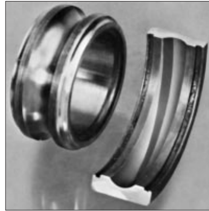
Examples of Bearings with Misaligned Rings
