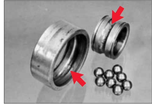
Flaking or Spalling of Raceway
