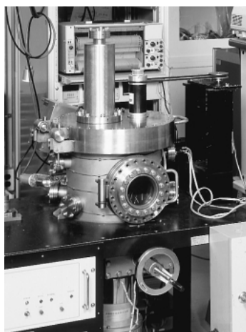
• 4-Ball type ultra-high vacuum test equipment
