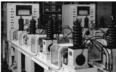
• Radial type life test equipment
