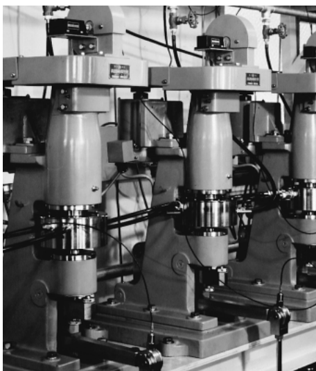
• Thrust type life test equipment
