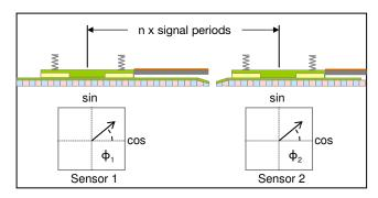
The AMSA 3L sensing system employs 2 sensors whose geometric spacing is precisely reflected in the geometry of the reading head. The sensors are cast into a special titanium slider housing.
