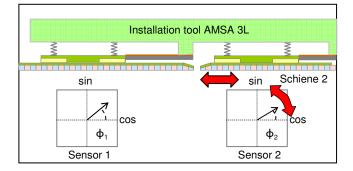
In conjunction with the installation software, the installation tool measures and displays the phase difference ( $\phi 2 - \phi 1$ ) so that the rail joint can be adjusted by moving the rails axially relative to each other. In the above example, the butt joint is adjusted by moving rail 2 in the direction of measurement until the phase difference is small enough; the mounting screws of the rail are then tightened in this position.
