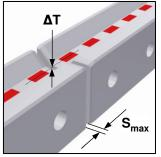
$\Delta T$  = Maximum height difference at the scale butt
