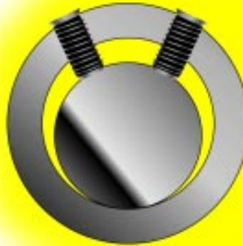
Set Screw Lock Shaft Displacement
