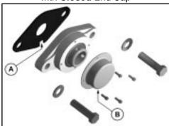
A: Drain Slot on Bottom
