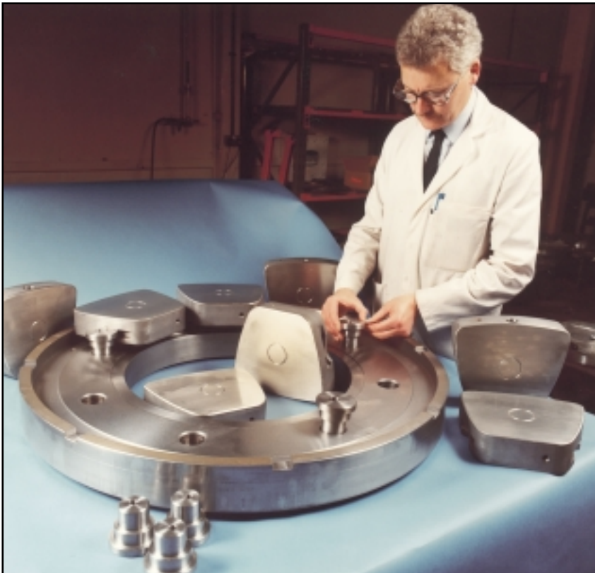
M8538/0 featuring high pressure jacking oil for start up and run down. Jacking oil annulus can be seen on the surface of each thrust pad.
